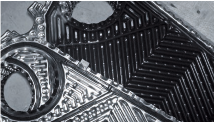
The centre of the temperature change: the cleaner the plates, cavities and gaps are, the better the medium in the heat exchanger can circulate.
